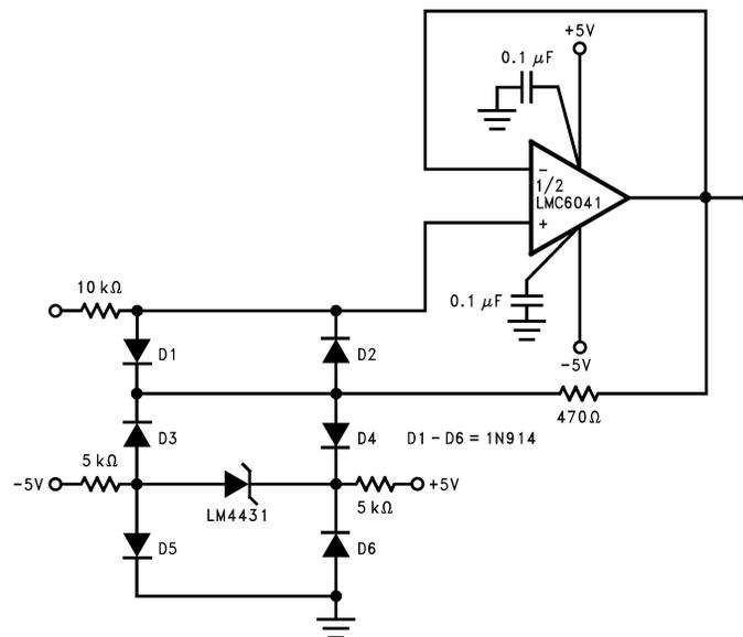
**Figure 10. Protecting Op amp input.**
