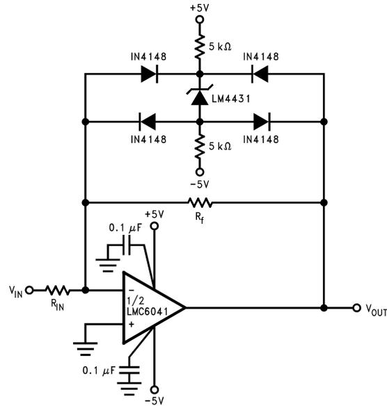
**Figure 9. Bounded amplifier reduces saturation-induced delays and can prevent succeeding stage damage.**
